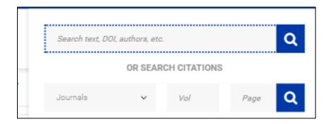
• SC 1.4.3 A – Color Contrast (Regular Text) – Search button text does not have minimum color contrast ratio of 4.5:1 against the inner background. It has color contrast ratio of 1.51:1
